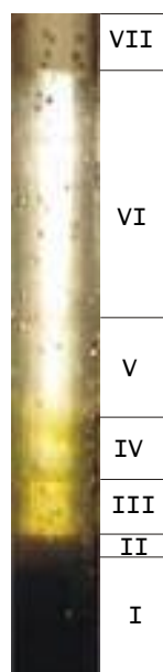
Figure 3. Fractionating of supercritical CO 2 -extracts of Salvia Officinalis L.
